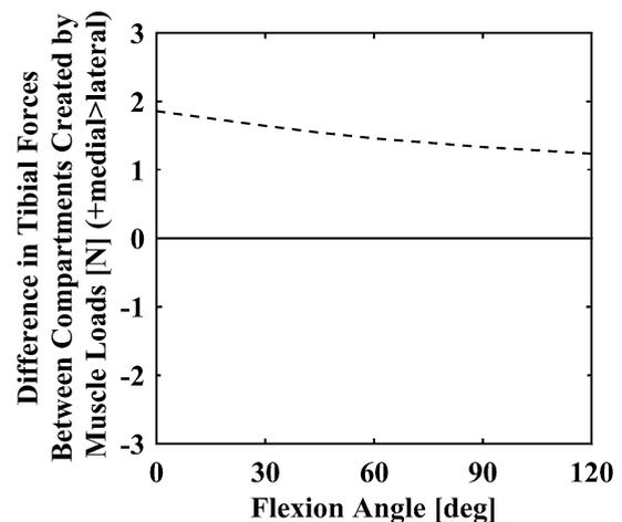
**Fig. 11** Line plot shows that applied muscle forces had a negligible effect on the differences in tibial forces between compartments from 0° and 120° of flexion measured in the present study
