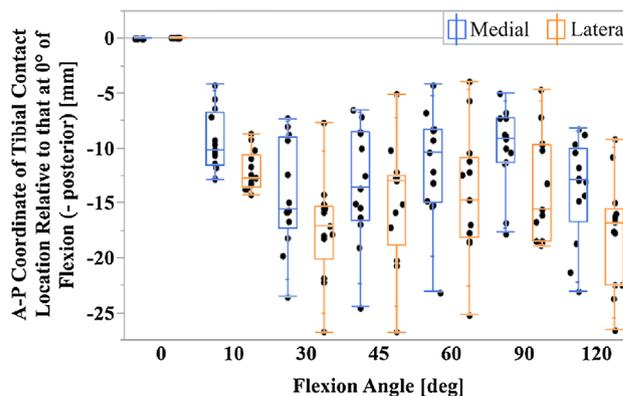
**Fig. 8** Box-and-whisker plot show the A–P coordinate of the contact location in each compartment during passive flexion from 0° to 120°. The lower and upper lines defining the box indicate the 1st quartile and the 3rd quartile, respectively, and the whiskers extend from the ends of the box to the outermost data point that falls within the distances computed as follows: 3rd quartile + 1.5 × (interquartile range) and 1st quartile − 1.5 × (interquartile range)
