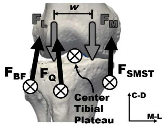
**Fig. 10** Coronal view of free body diagram of the knee with applied muscle loads
