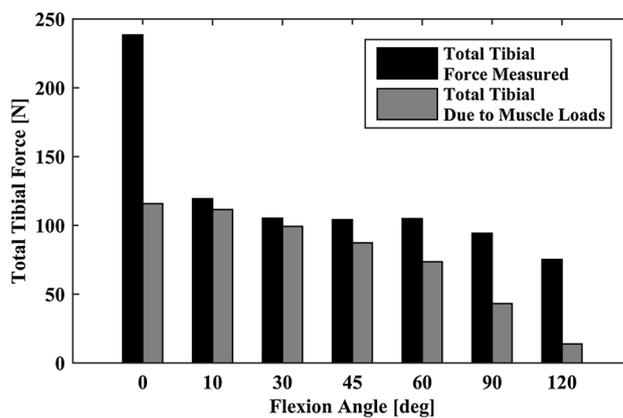
Fig. 14 Vertical bar graph shows the average total tibial force measured and the compressive force component of the applied muscle loads
