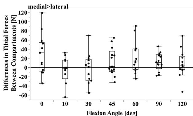
**Fig. 7** The box-and-whisker plot shows the differences in tibial forces between compartments for each of the thirteen KA TKAs at each flexion angle. The lower and upper lines defining the box indicate the 1st quartile and the 3rd quartile, respectively, and the whiskers extend from the ends of the box to the outermost data point that falls within the distances computed as follows: 3rd quartile + 1.5 × (interquartile range) and 1st quartile − 1.5 × (interquartile range)
