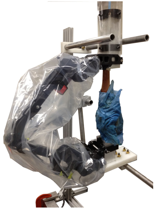
Figure 3. A photograph of the motion application fixture with a knee specimen at full extension with the ISL attached.
