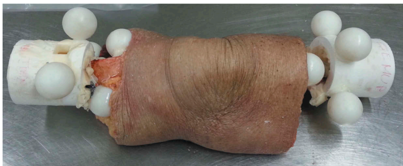
Figure 1. Knee specimen after potting and application of the fiducial markers.
